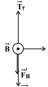
$$F'_{\text{net}} = 0 \Rightarrow T_2 = F'_B + W \quad (2)$$
